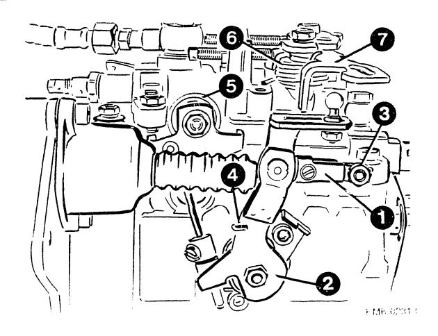
ADJUSTING TEMPERATURE—DEPENDENT IDLE INCREASE ACTING ON HOUSING—FIXED IDLE SPRING
